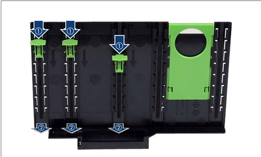
Figure 72: Removing the engaging hooks
